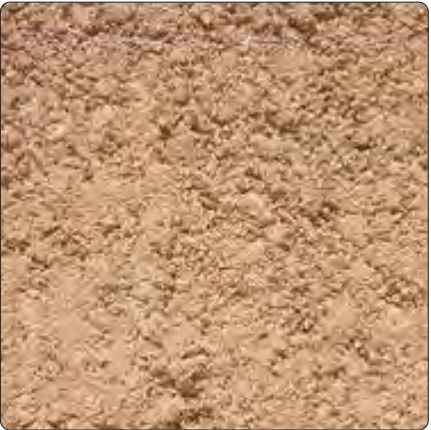
GraniteCrete Permeable aggregate surfacing Natural stone with proprietary binder "Desert Sand"
